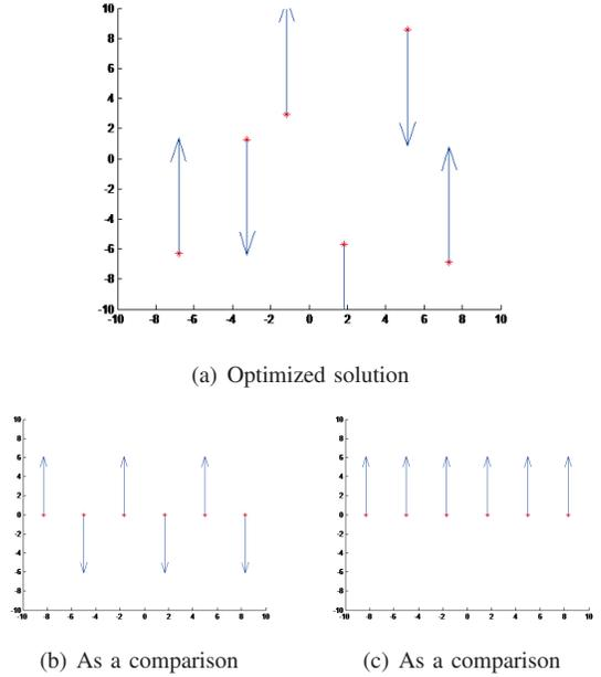
Fig. 2. In the first environment, the initial locations and heading directions of gliders in (a) are optimized by GA method, while as comparison, (b) and (c) are following intuitive distribution.
