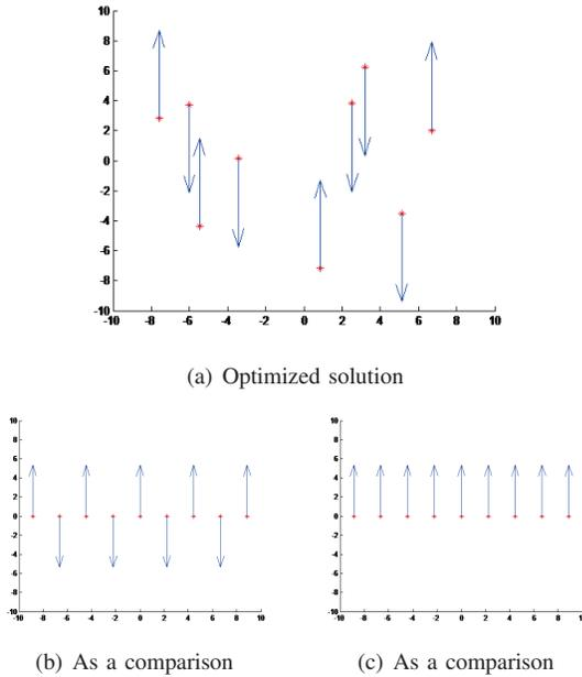
Fig. 4. In the second environment, the initial locations and heading directions of gliders in (a) are optimized by GA method, while as comparison, (b) and (c) are following intuitive distribution.
