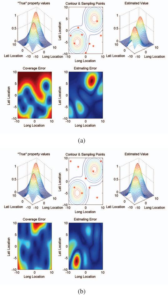
Fig. 5. Two snapshots of observation state of gliders moving along transects. From left to right, up to bottom sequentially are the value of generated scalar field, locations of gliders, estimated value, coverage error (uncertainty) and estimating error.
